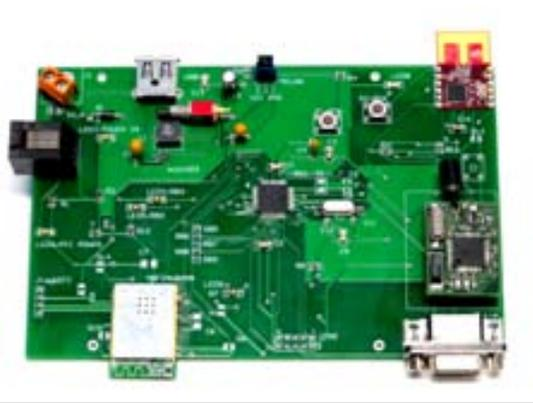
Figure 4. Cognitive Wireless Sensor Network Device prototype
