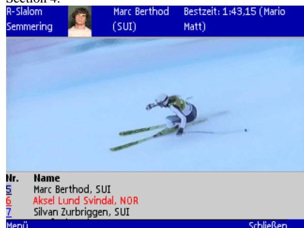
Figure 9: iTV Split-screen View on a Nokia E61 Symbian Device based on two Browser- and one Video Panel.
