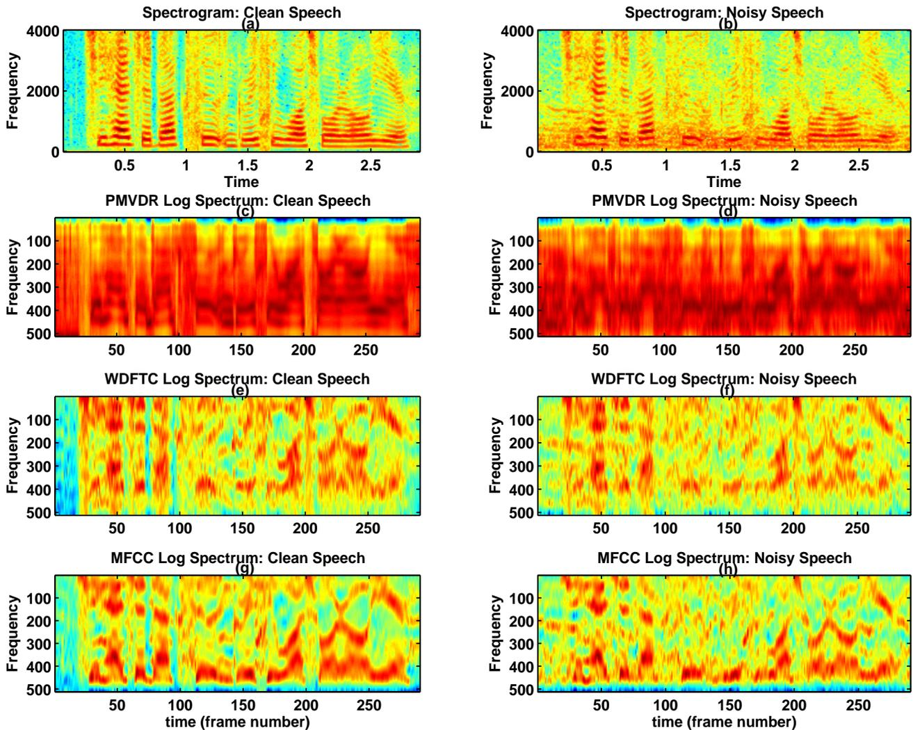
Figure 2. Illustrating the impact of 5 dB babble noise on PMVDR, WDFTC and MFCC Log spectra: (a) Spectrogram of clean speech, (b) Spectrogram of noise corrupted speech (a), (c) PMVDR log spectrum of clean speech (a), (d) PMVDR log spectrum of noise corrupted speech (a), (e) WDFTC log spectrum of clean speech (a), and (f) WDFTC log spectrum of noise corrupted speech (a), (g) MFCC log spectrum of clean speech (a), and (h) MFCC log spectrum of noise corrupted speech (a).
