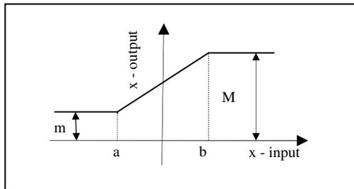
**Figure 10. Saturation Non-Linearity**
