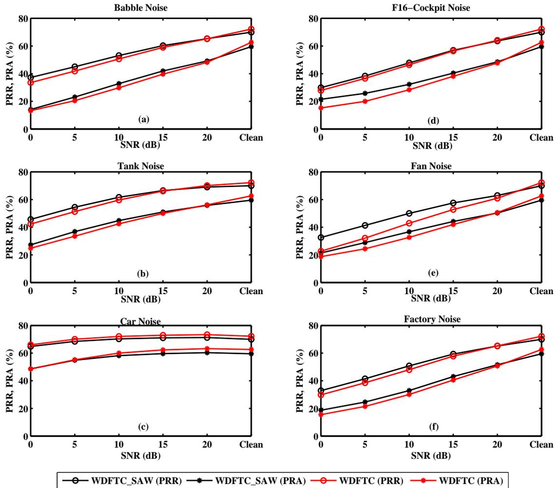
Figure 7. Illustrating the impact of different noises at various SNRs on WDFTC and WDFTC\_SAW phoneme recognition rate (PRR) and phoneme recognition accuracy (PRA): (a) babble, (b) tank, (c) car, (d) F-16 cockpit, (e) fan, and (f) factory noises. Acoustic Models trained on speech samples from a male speaker in the TIMIT corpus using diagonal (DC) covariance.
