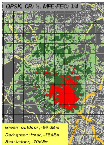
Figure 9. The predicted coverage area for QPSK, with the raster size of 1.6 km.
