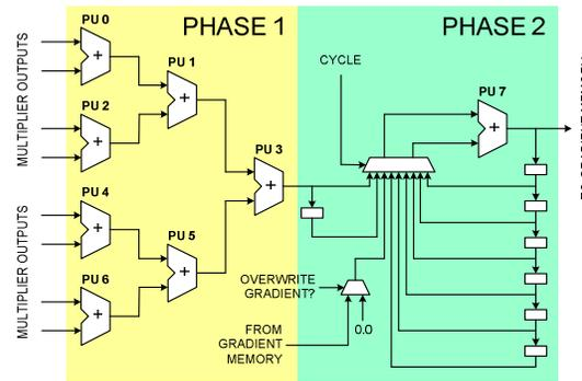
Fig. 9. Adder tree pipeline stages.
