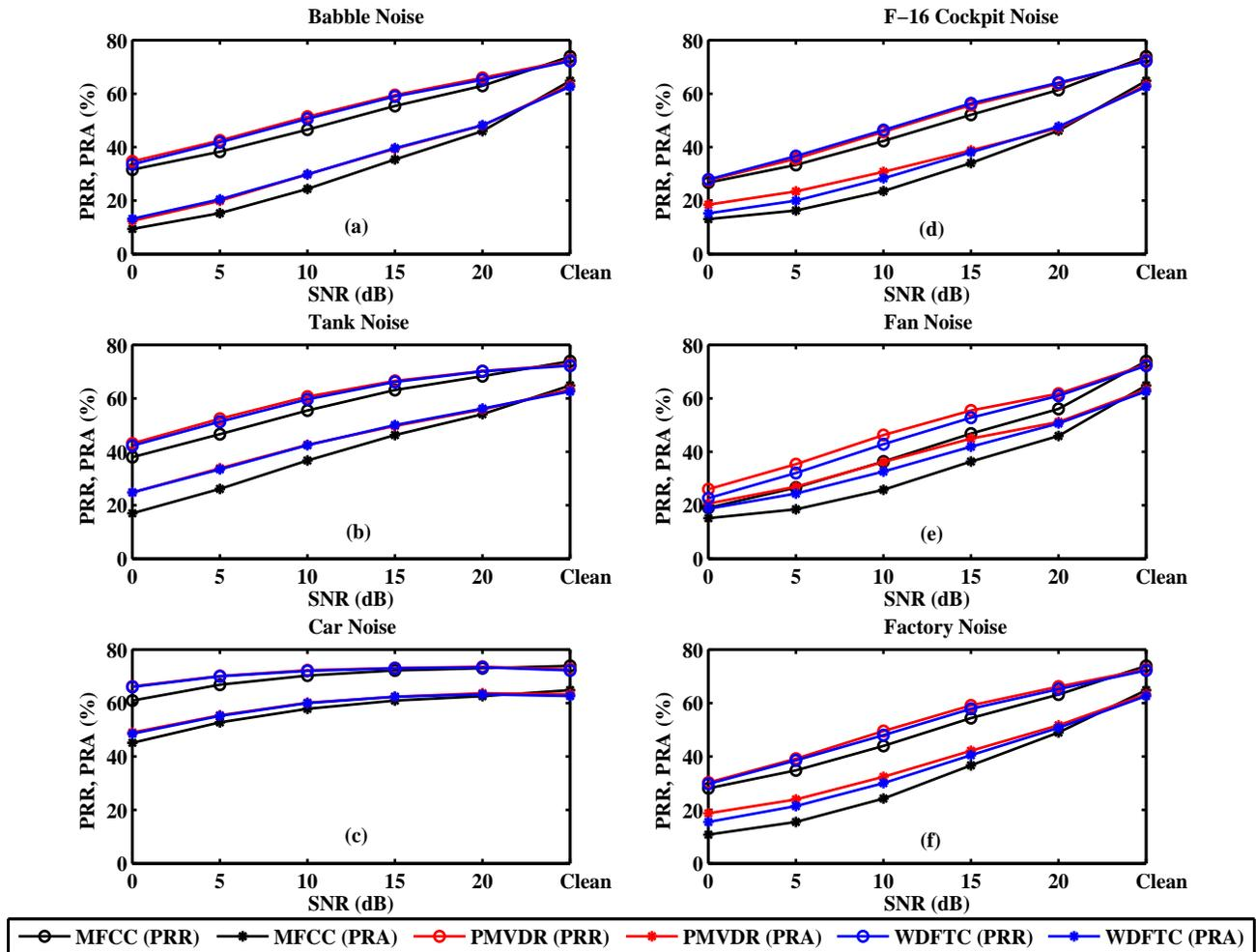
Figure 4. Illustrating the impact of different noises at various SNRs on MFCC, WDFTC and PMVDR phoneme recognition rate (PRR) and phoneme recognition accuracy (PRA): (a) babble, (b) tank, (c) car, (d) F-16 cockpit, (e) fan, and (f) factory noises. Acoustic Models trained on speech samples from a male speaker in the TIMIT corpus using diagonal (DC) covariance.
