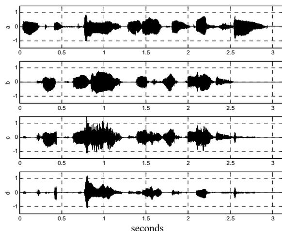
Fig. 9. Performances of the NLMS algorithm for speech signals, during double-talk: (a) far-end signal  $x(n)$ ; (b) near-end signal  $u(n)$ ; (c) recovered near-end signal in  $e(n)$ ; (d) residual error  $r(n)$ .
