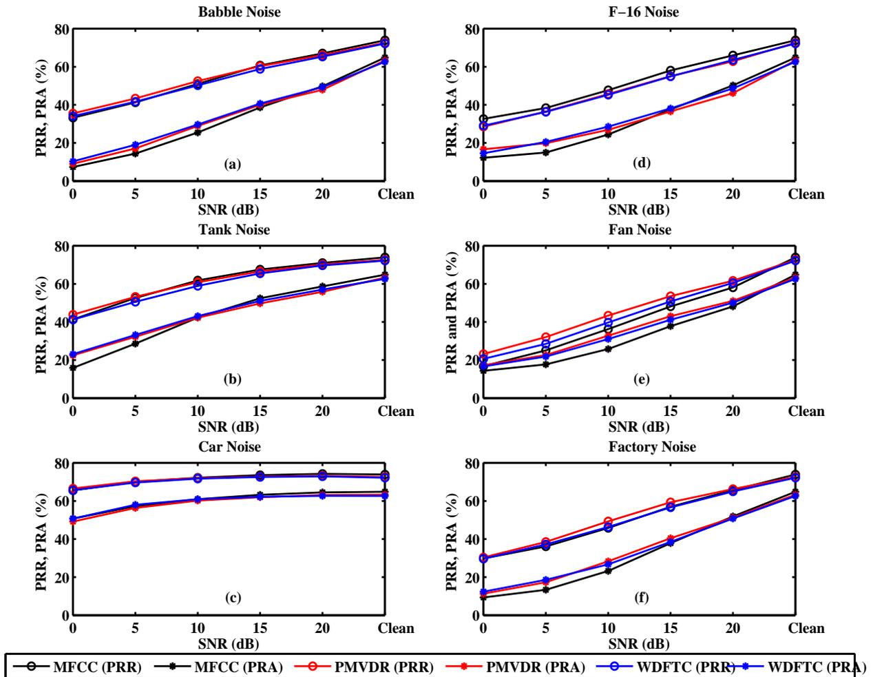
Figure 5. Illustrating the impact of different noises at various SNRs on MFCC, WDFTC and PMVDR phoneme recognition rate (PRR) and phoneme recognition accuracy (PRA): (a) babble, (b) tank, (c) car, (d) F-16 cockpit, (e) fan, and (f) factory noises. Acoustic Models trained on speech samples from female speaker in the TIMIT corpus using diagonal (DC) covariance.
