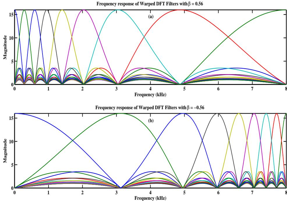
Figure 1. 16-Band Warped Filter bank shown for  $f_s/2$ . (a)  $\beta = 0.56$  (b)  $\beta = -0.56$
