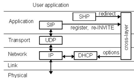
Fig 7. Protocol Stack at Mobile Node.
