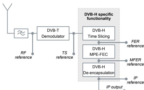
Figure 5. A principle of the reference DVB-H terminal.
