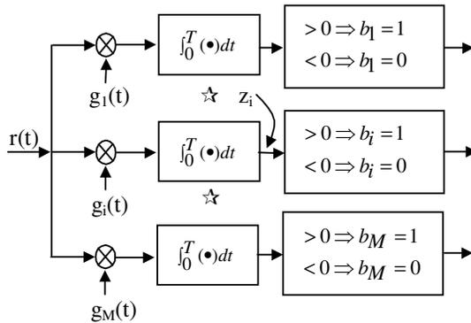
Figure 2. fm Receiver for orthogonal functions
