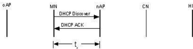
Fig. 9. Address allocation with DHCP-FCLH.
