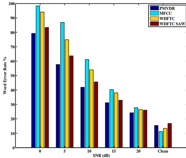
Figure 9. Word Error Rate (WER) of MFCC, PMVDR, WDFTC and WDFTC\_SAW features under noise-free and Babble noise conditions
