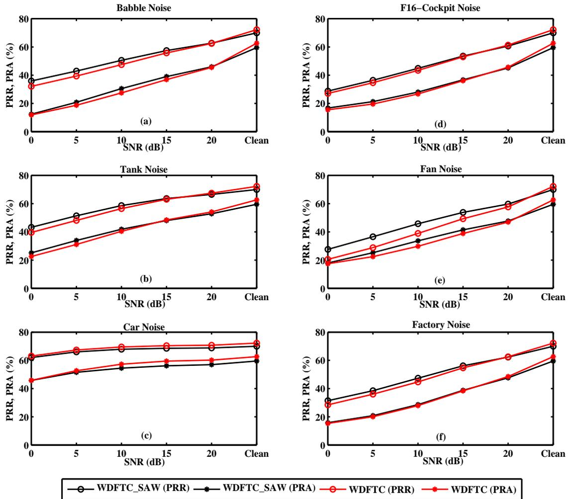
Figure 6. Illustrating the impact of different noises at various SNRs on WDFTC and WDFTC\_SAW phoneme recognition rate (PRR) and phoneme recognition accuracy (PRA): (a) babble, (b) tank, (c) car, (d) F-16 cockpit, (e) fan, and (f) factory noises. Acoustic Models trained on the entire TIMIT corpus using diagonal (DC) covariance.
