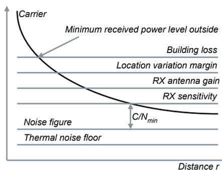
Figure 26. The main principle of the DVB-H link budget.
