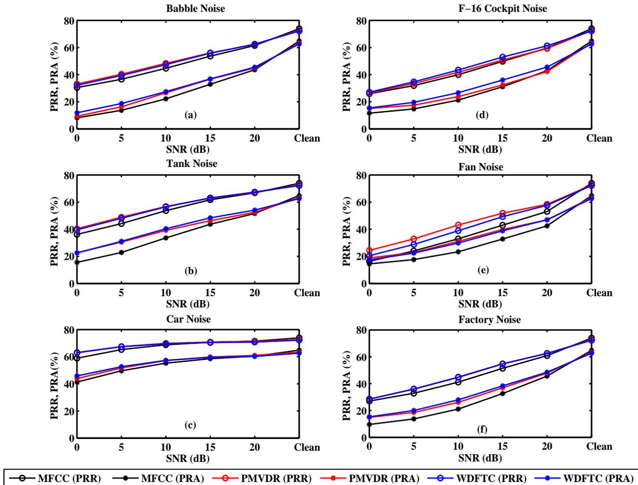
Figure 3. Illustrating the impact of different noises at various SNRs on MFCC, WDFTC and PMVDR phoneme recognition rate (PRR) and phoneme recognition accuracy (PRA): (a) babble, (b) tank, (c) car, (d) F-16 cockpit, (e) fan, and (f) factory noises. Acoustic Models trained on the entire TIMIT corpus using diagonal (DC) covariance.
