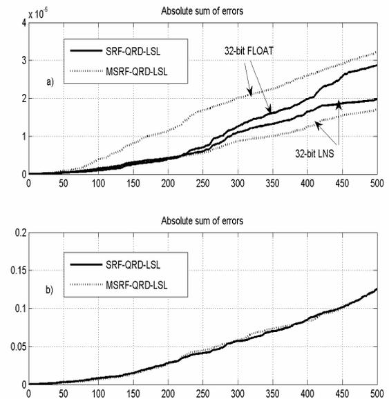
Fig. 4. (upper) The absolute sum of errors for 32-bit LNS and FLOAT implementations of the investigated algorithms; (lower) The absolute sum of errors for 20-bit LNS implementations of the investigated algorithms.
