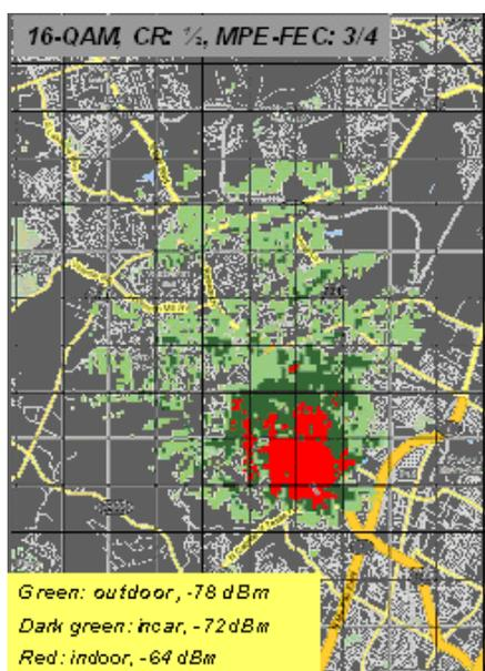
Figure 8. The predicted coverage area for 16-QAM. The raster shown in the map is 1.6 km. The main lobe and the test route is to north-west direction from the site.
