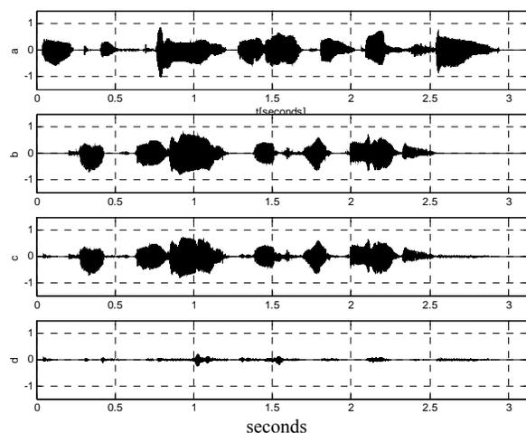
Fig. 10. Performances of the MSRF-QRD-LSL algorithm for speech signals, during double-talk: (a) far-end signal  $x(n)$ ; (b) near-end signal  $u(n)$ ; (c) recovered near-end signal in  $e(n)$ ; (d) residual error  $r(n)$ .
