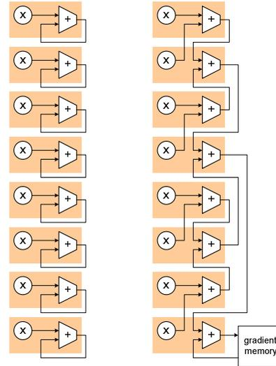
Fig. 8. Left: normal configuration. Right: Adder tree configuration.
