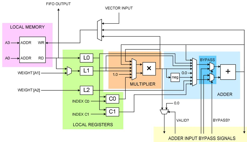
**Fig. 6. RTL description of a processing unit.**
