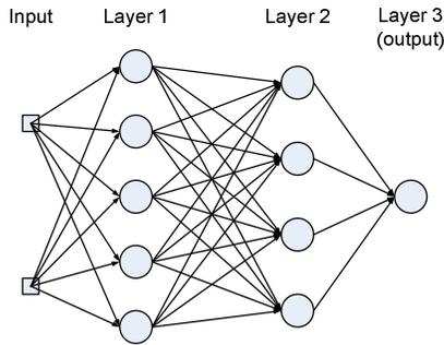
**Fig. 1. A fully connected 2/5/4/1 multilayer perceptron.**
