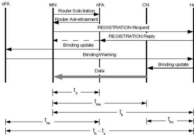
Fig. 2. Handover process in Mobile IP with RO.
