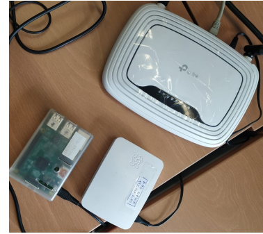
(c) Physical scenario, including a wireless router and 2 raspberry pis.
