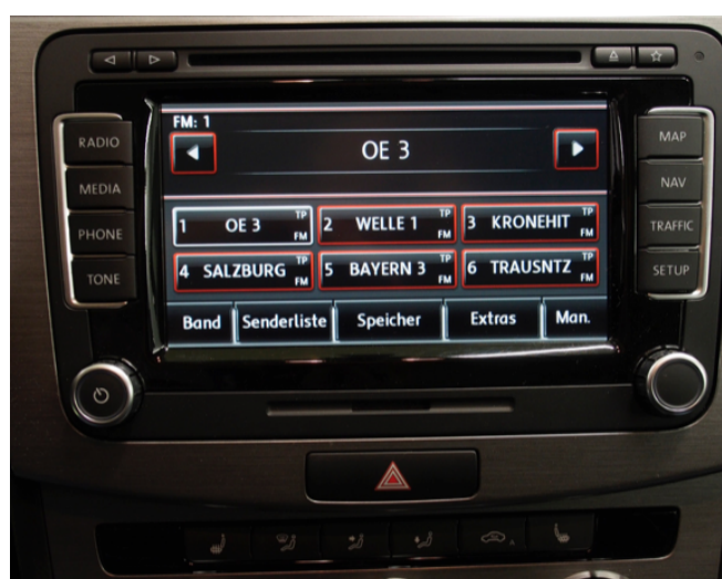
Figure 10. VW Passat dashboard which combines few physical buttons with a well-readable touch display.
