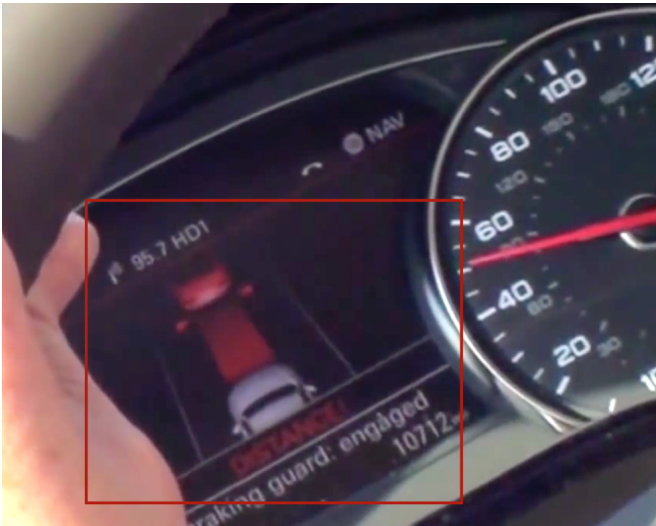
Figure 5. Audi A8 Distance Warning through a combination of auditory and visual warning displays.
