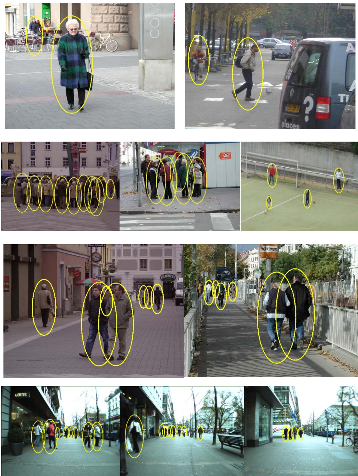
Figure 18. First three rows shows the results obtained from INRIA database and fourth row shows some results from ETH pedestrian database. The performance of our detector in occlusions, cluttered scenes, and pose variations, should be noted.
