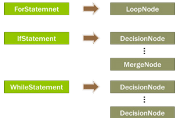
Figure 8. From AST to intermediate representation.
