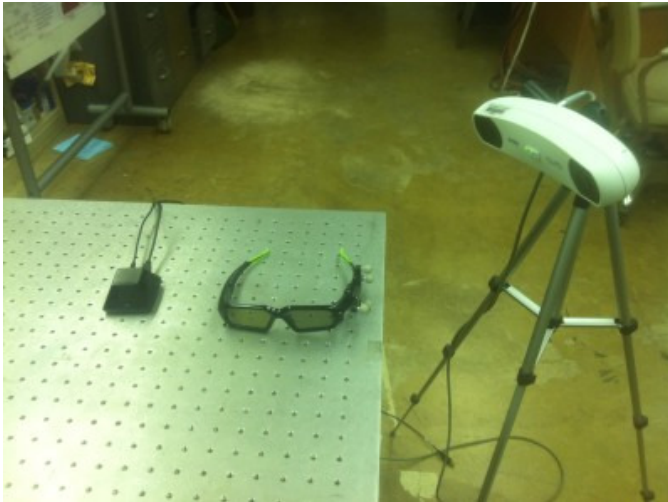
Figure 4: Shutter glasses with synchronization signal transmitter, reflective markers, and localizer for 3D graphic display with head tracking
