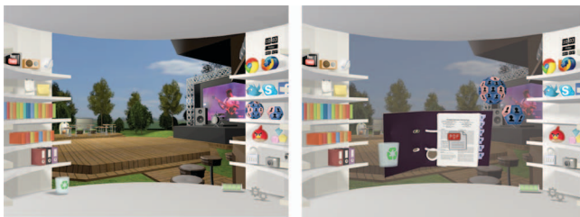
Figure 7. The finalized design of Room GUI. On the left start view and on the right target objects (trashcan and contact balls) provided when a copy has been made.
