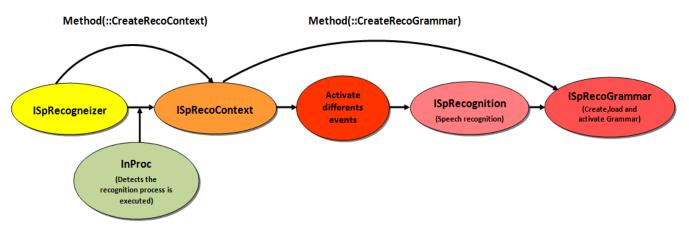
Figure 4. Windows interface execution thread.
