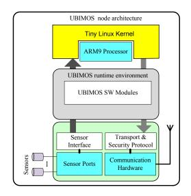
Figure 2. The structural organization of the wearable computer used as UAs and IMPs
