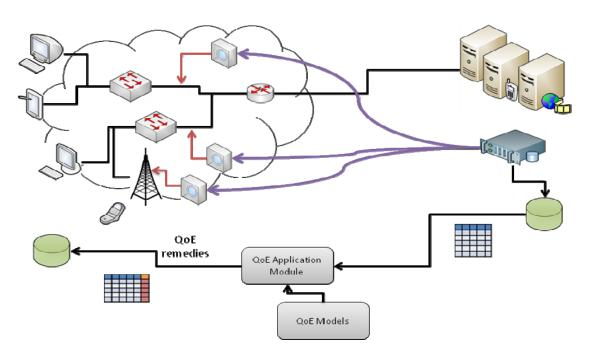
Figure 4. QoE estimation and remedies architecture
