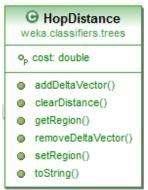
Figure 7. HopDistance class diagram
