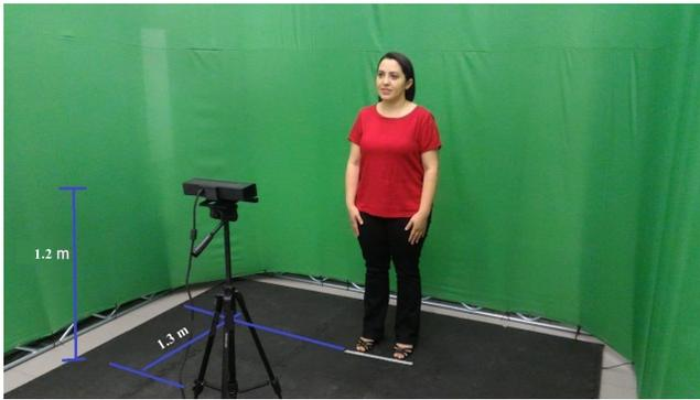
Fig. 2. Positioning and relative distances of the signer to the device.
