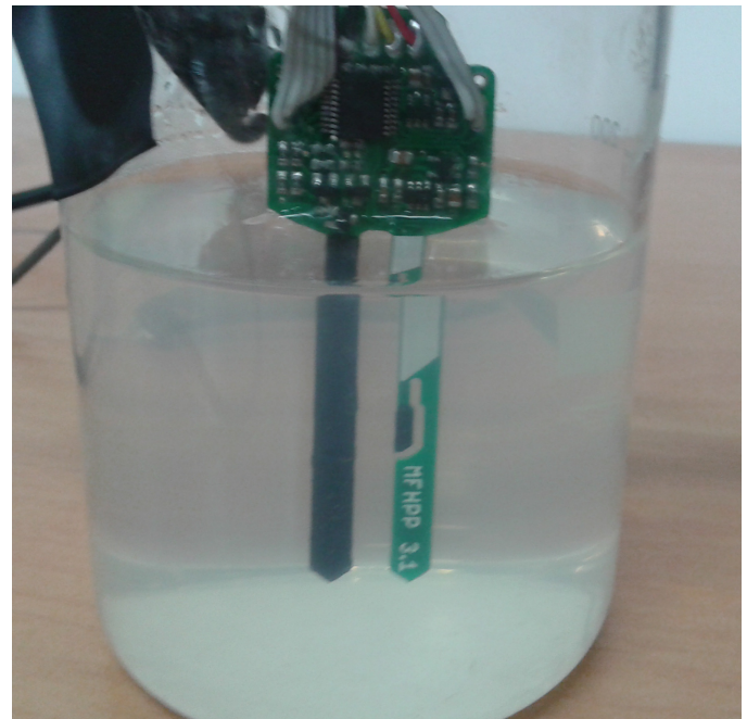
Figure 6. Probe distance calibration in agar solution
