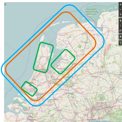
Figure 12. Locations of the Wadden Sea shown on OpenStreetMap; the TerraSAR-X footprints are in green, the Sentinel-1A footprint is in orange, and the Sentinel-2A footprint (all quadrants) is in blue.
