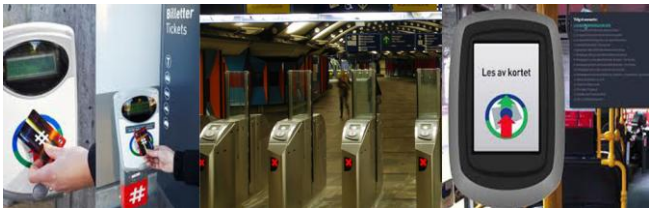
Figure 2. Smart card ticket readers at metro stations and on the bus.
