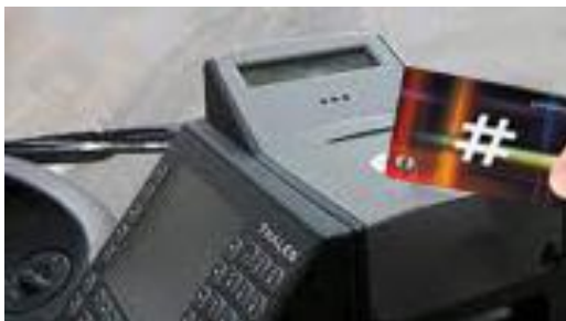
Figure 5. Validating a smart card ticket on the bus.
