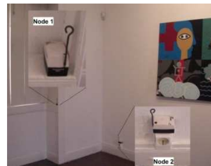
Fig. 6. Wireless Sensor Network deployment in an exposition room of Fortaleza São Tiago
