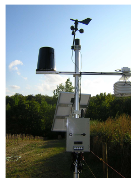
Figure 8. VineSense GPRS Gateway with Weather Sensors.
