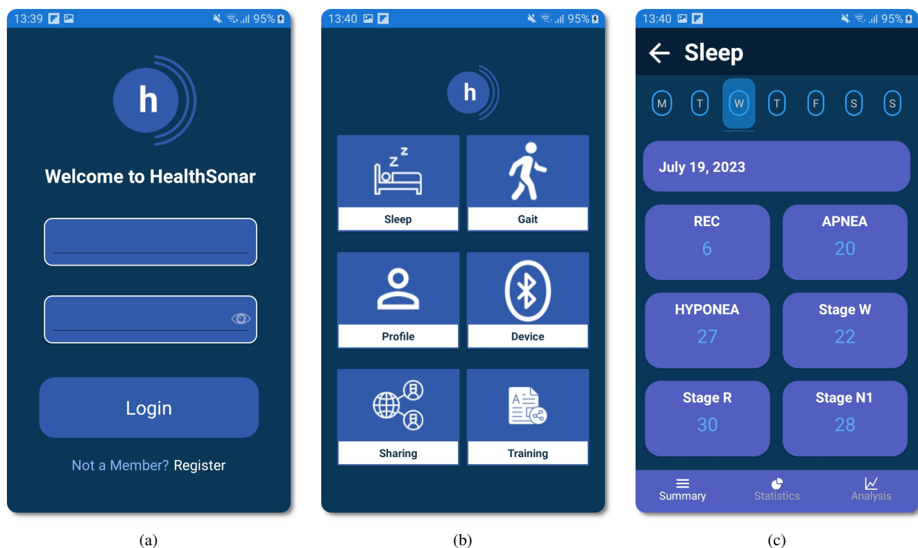
Fig. 4: Various screens of the HealthSonar mobile application. (4a) The login screen. (4b) The main menu. (4c) The sleep analytics. The app provides a user-friendly interface to the HealthSonar system, assisting users in configuring the device before its first use, as well as providing sleep metrics, sleep-related events, mobility metrics and real-time fall notifications.
