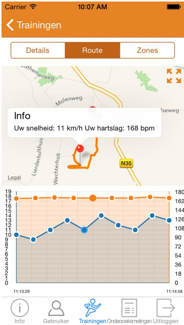
Figure 10. Detailed training overview zoomed in. Left scale and blue line: speed (km/h); Right scale and orange line: heart rate (bpm). When tapping a measuring point in the diagram, the location at that point is shown on the map by the red bullet. You can also see the speed and heart rate at that point.
