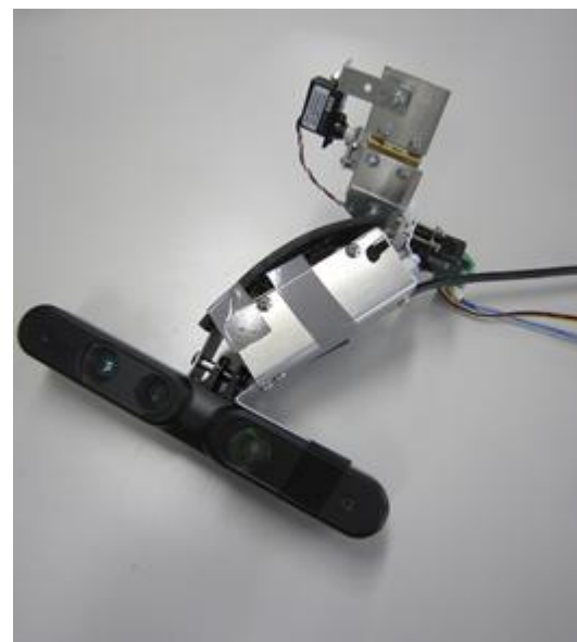
Figure 11. Prototype of FB-Finger2, designed with 2-degrees-of-freedom.
