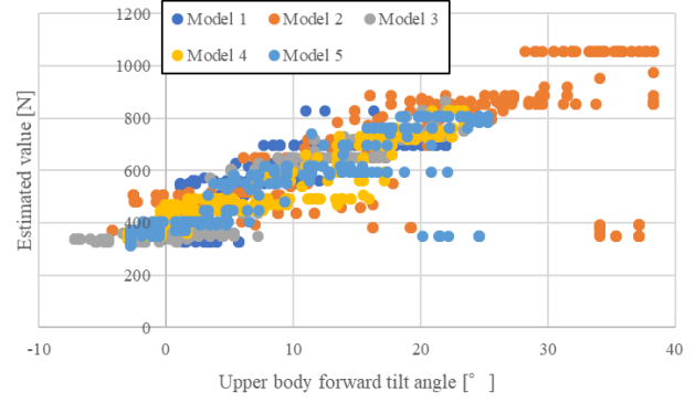
Figure 7. Intervertebral disc compression forces estimated for untrained persons by deep learning models trained on multiple people for each anterior tilt angle. For example, Model 1 plots the results of a deep learning model created with participants B, C, D, and E as training data, with participant A estimated as validation data.
