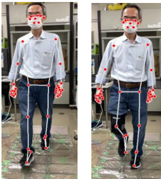
Figure 3. Skeleton analysis of motion (a) without and (b) with restrictions using video from front.
