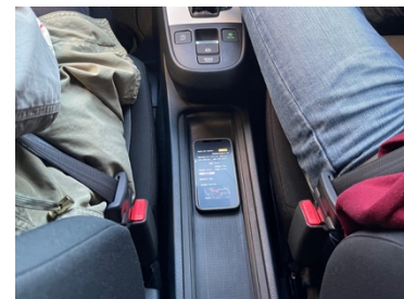
Figure 4. Measurement of vehicle speed and angular velocity using smartphone sensors
