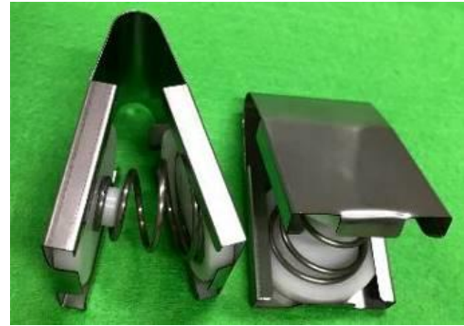
Figure 11. Two views of the spring assist unit (heel-up spring).
