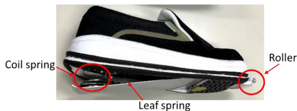
Figure 6. Assist shoe prototype.
