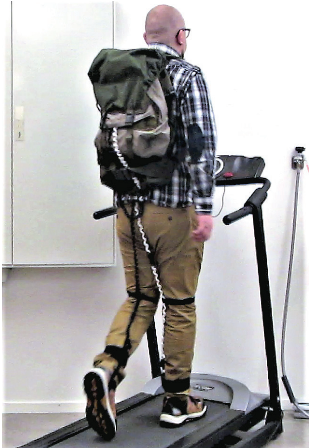
Figure 6. Walk on treadmill with backpack containing the electronics of the IngVaL system and the extra carried weights.
