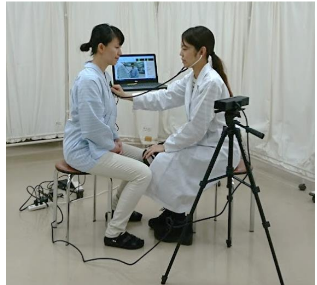
Figure 6. The KINECT-Based Auscultation Practice System (Face-to-face arrangement)
