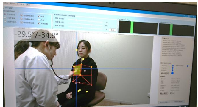
Figure 7. The KINECT-Based Auscultation Practice System (Screen of control computer)
