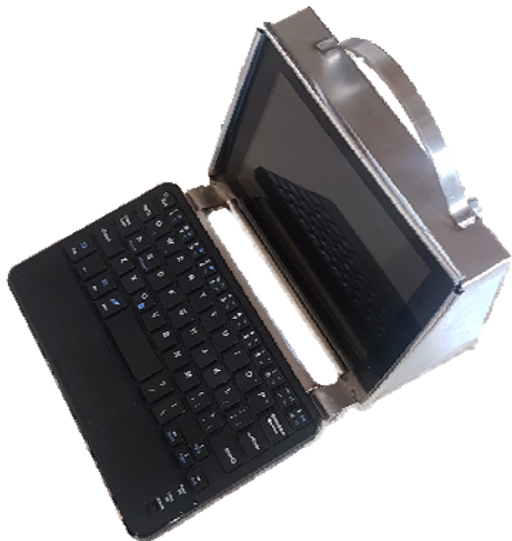
Figure 12: Portable central unit based on Raspberry Pi
