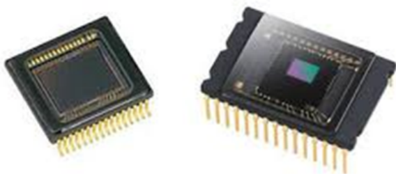
Figure 4. Example of CCD (left) and CMOS (right) sensor [21].
