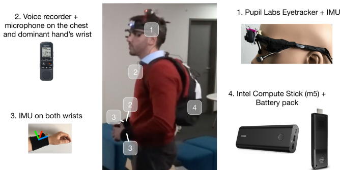
Figure 1. Recording setup for each participant includes an eyetracker connected to a small recording computer. Additional sensors: IMU on both arms and head, microphone on the wrist and at the chest.
