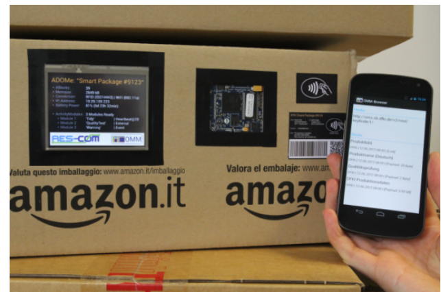
Figure 11. Performing built-in and on-product integrity checks on a smart package equipped with ADOMe and accessed by a mobile handheld device.
