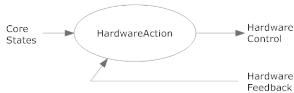
Figure 11: The Action Entity “HardwareAction”
