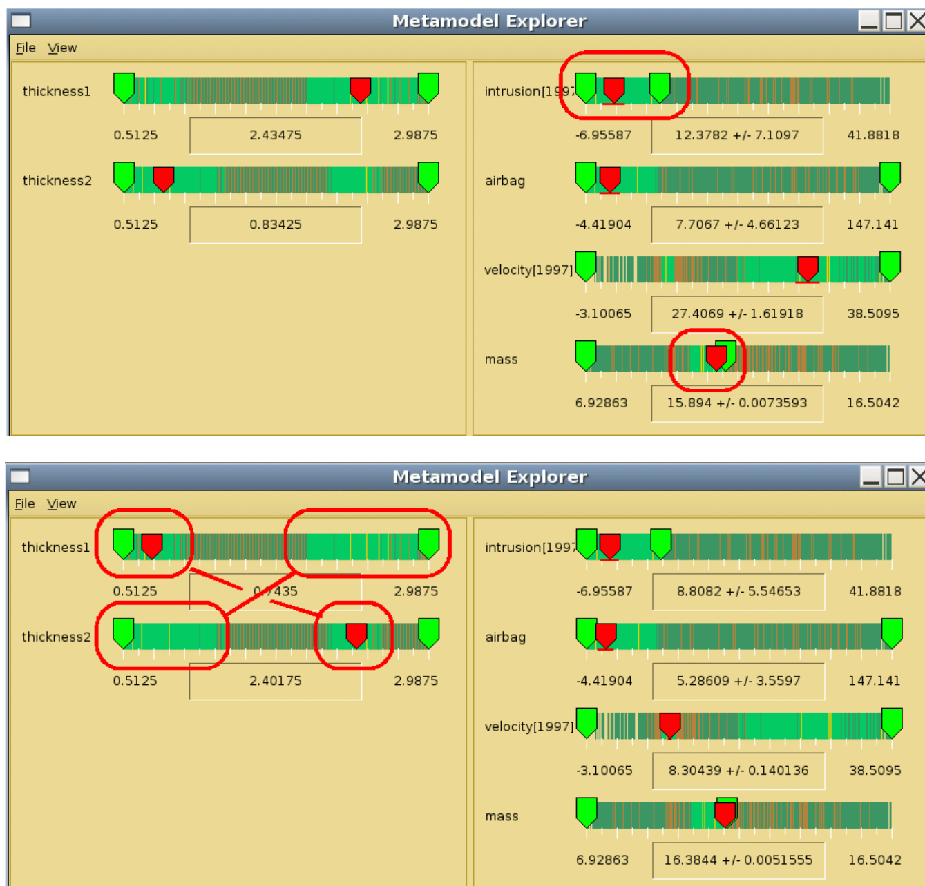
Figure 6. Studying Audi B-Pillar crash test in DesParO Metamodel Explorer. Top: an attempt to minimize simultaneously intrusion and mass by setting upper constraints on these criteria. Bottom: two islands of available solutions become visible.
