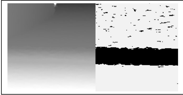
Figure 2. Left side: Depth values from the Sensor in grayscale (White near, dark grey far away) with a 10 mm tread in a distance of 80 cm, right side: Visualization after ground subtraction and converted to a binary image of depth values with the RMS as threshold.
