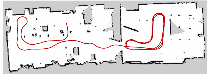
Figure 8. Occupancy grid map from SLAM approach and the smoothed travelled path
