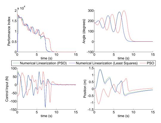
Fig. 5. Unconstrained nonlinear MPC: A comparison
