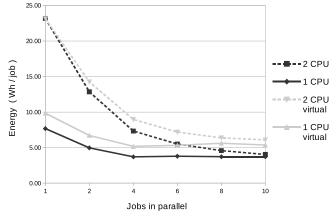
Figure 17. Energy consumption per job with different number of virtual machines running one job each
