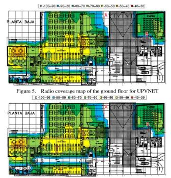
Figure 7. Radio coverage map of the ground floor for EDUROAM
