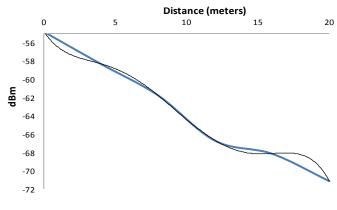
Figure 17. Average signal strength on the ground floor
