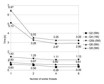
Figure 8. The speed up obtained by implicit parallelization
