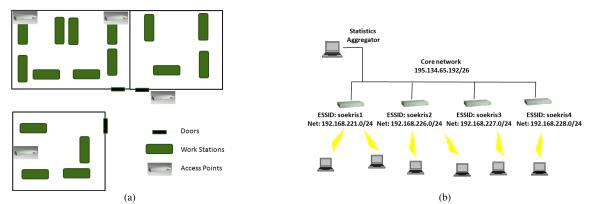
Figure 8: (a) Physical topology of the experimentation environment, (b) network topology of the experimentation environment.
