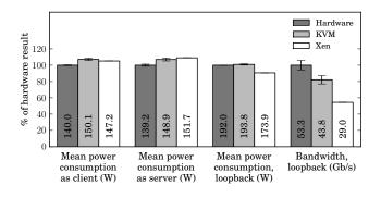
Figure 8. Power consumption under Iperf network traffic test
