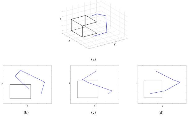
Figure 5. An example of 3D trajectory (a) and its projections on the different coordinate planes xy (b), xt (c) and yt (d). Although the trajectory does not intersect the query box, its projections do it.
