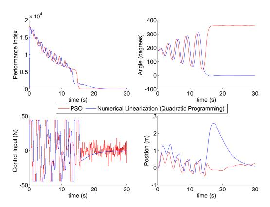
Fig. 6. Constrained nonlinear MPC: Restricting control input to within -45N and 45N (10 independent trials)
