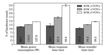
Figure 12. The effect of workload on virtual machine performance with KVM using different virtual machine resources
