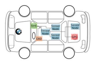
Figure 5: Measurement system - All data from the sensor nodes and the GPS module is transmitted to the data sink in the vehicle
