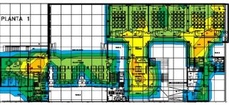
Figure 10. Radio coverage map of the first floor for EDUROAM
