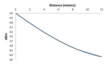
Figure 19. Average signal strength on the second floor
