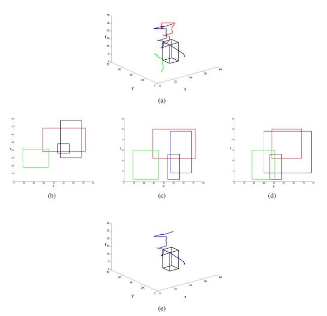
Figure 6. An overview of the method. (a) a query box and three trajectories; (b), (c), (d): the projections of trajectories' MBRs on the coordinate planes; (e) the final result of our method, after the application of the clipping algorithm on the blu and red trajectories.
