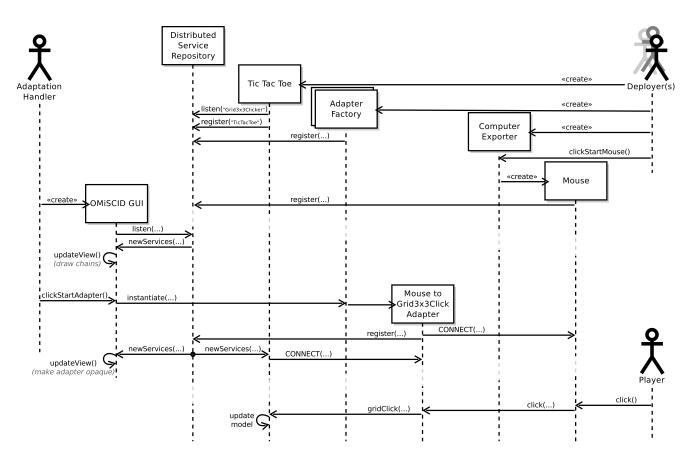
Figure 6. Sequence diagram showing the interactions between different parts of the system. First, the application and some base services are deployed, then the adaptation layer is populated and finally the player plays a turn. Only one input is provided, no display/output for the game is shown in this diagram. See Section V-B for details.
