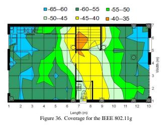
For our comparison, we should observe the signal propagation through the walls, as it can be found in any building.
