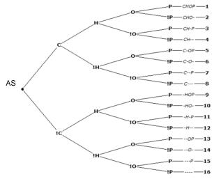
Figure 2: Combination of autonomic functionalities (for n = 4).
