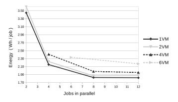
Figure 19. Energy consumption per job in virtual machines when varying resources and job parallelism
