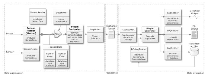
Figure 4: GREASE framework structure which allows the strict separation into two operation phases (measurement and evaluation)
