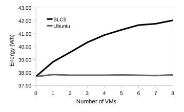
Figure 4. Energy consumption of idle virtual machines
