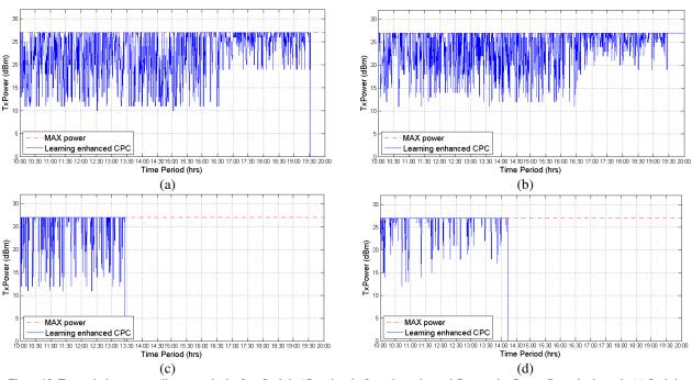
Figure 12: Transmission power adjustments in the four Soekris APs using the Learning enhanced Cooperative Power Control scheme in (a) Soekris AP1, (b)Soekris AP2, (c)Soekris AP3, (d)Soekris AP4
