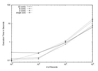
Figure 5. Comparison of execution times for bulk pattern recognition depending on the number of reading for different number of CPU cores.
