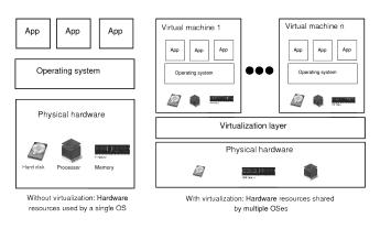
Figure 1. A non-virtualized and a virtualized system
