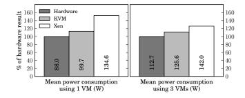
Figure 9. Power consumption of different virtualization solutions with different number of virtual machines in the repository test
