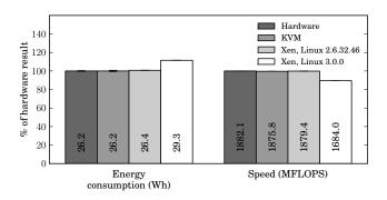
Figure 7. Energy consumption under high CPU load with Linpack
