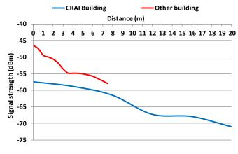
Figure 37. Signal strength for the IEEE 802.11g
