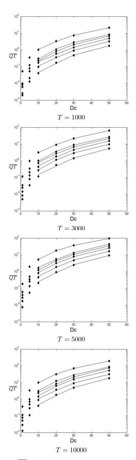
Figure 12.  $\overline{QT}$  (in seconds) as the dimension of the querying cube (in percentage of the whole volume) increases and having *L* as parameter.
