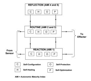
Fig. 1. An Autonomic Computing expression of the IMD (The AMI is discussed at length in Section III)
