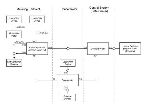
Figure 1. FMC Illustration of Advanced Metering Infrastructure, as defined in [13].
