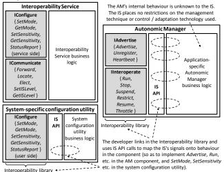
Figure 3. Internal architecture of the system components and the integration of the IS interfaces with these components.
