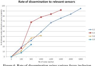
Figure 6. Rate of dissemination using various fuzzy inclusion thresholds
