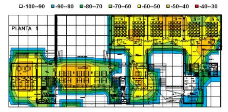
Figure 23. Estimated signal strength on the first floor for the proposed AP relocation.
