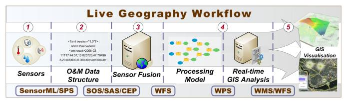
Figure 4. Live Geography - Standardised Geo-Sensor Data Analysis Architecture.
