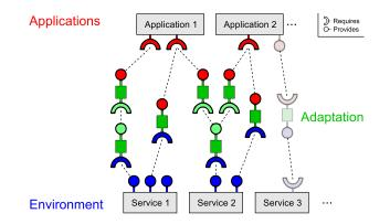
Figure 3. Proposed EAA architecture – *Environment* provides low-level services. *Applications* manipulate only high-level abstract services. *Adaptation* bridges the two and is dynamically extensible and user-controlled. Lighter chain on the right: inversion due to the whiteboard pattern.
