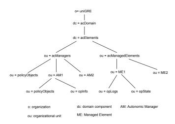
Fig. 24. Example DIT for an Autonomic Computing System
