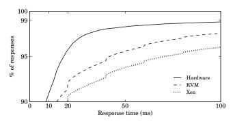
Figure 13. The impact of virtualization solution on quality of service
