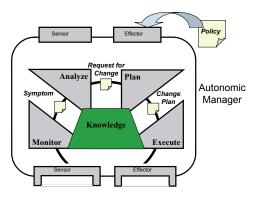
Fig. 1. IBM Autonomic MAPE Architecture [5]
