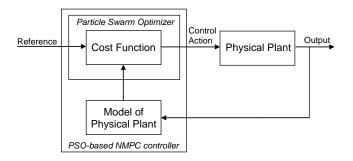
Fig. 2. PSO-based nonlinear MPC loop
