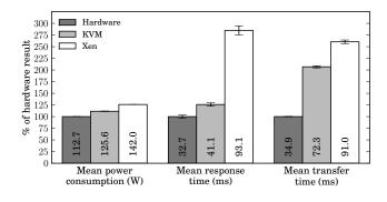
Figure 10. Power consumption and Httperf results of different virtualization solutions
