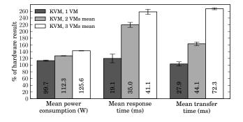
Figure 11. The effect of workload on virtual machine performance with KVM using different amounts of virtual machines
