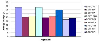
Figure 5. ICT energy savings compared to un-optimized, generally used RR with FIFO, BFF, and BBF  $\,$
